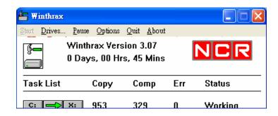
Step 3. Run Winthrax under chamber temperature of 25°C, 35°C, 40°C, and 45°C. Record the Hard Disk temperature of each time stamp and each room temperature by the thermal testing device.
